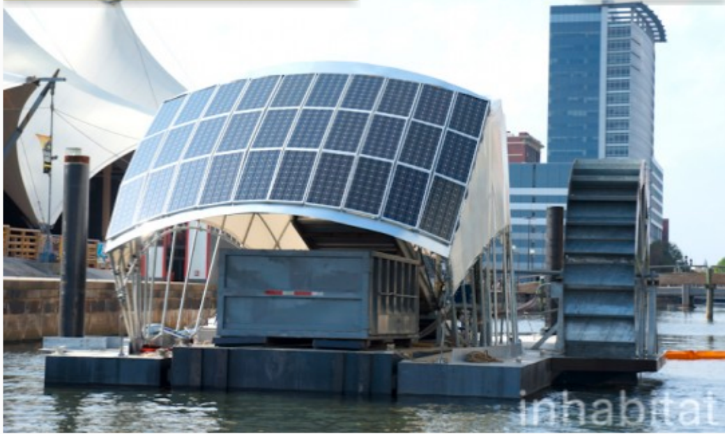
Trash isn't a pretty sight, but Baltimore's new Water Wheel actually makes collecting garbage look cool and fun. Powered by 30 solar panels and the water current, the Water Wheel Trash Inceptor can remove a whopping 50,000 pounds of trash a day—a rate that the Waterfront Partnership of Baltimore hopes will make the harbor swimmable by 2020. Designed by Clearwater Mills' John Kellett and Daniel Chase, the solar-powered trash collector generates 2,500 watts of electricity a day, which is enough energy to power the average Maryland home.
